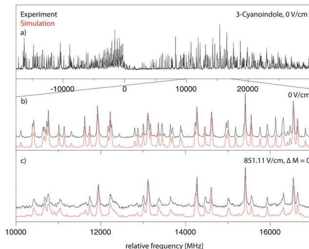
Fig. 4 Rotationally resolved electronic spectrum of the electronic origin of 3-cyanoindole at zero field and at 851.11  $\text{V cm}^{-1}$  with  $\Delta M = 0$  selection rules, along with a simulation with the best CMA-ES fit parameters.
