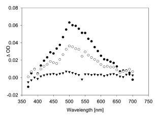
Fig. 4 Transient spectra, observed upon LFP ( $\lambda_{\rm exc}$  = 355 nm, 120 mJ per pulse) of 7 (0.1 mM) in benzene, purged with argon. Black circles: 14 ns after LFP. White circles: 34 ns after LFP. Black triangles: 150 ns after LFP.
