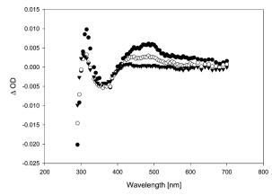
Fig. 3 Transient spectra, observed upon LFP ( $\lambda_{exc}$  = 355 nm, 120 mJ per pulse) of 7 (0.1 mM) in benzene, purged with argon. Black circles: 400 ns after LFP. White circles: 3.4 µs after LFP. Black triangles: 15 µs after LFP.
