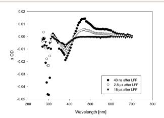
Fig. 2 Transient absorption spectra, monitored after different time intervals following LFP ( $\lambda_{exc}$  = 355 nm, laser attenuated to ca. 20 mJ per pulse) of a 0.1 mM solution of 8 in benzene, purged with argon
