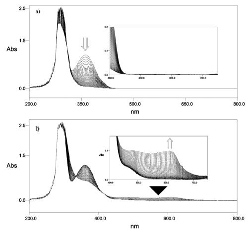
Fig. 1 UV-vis changes observed upon photolysis of Barton ester 7 (490 μM), (a) in dry benzene containing TFA (490 μM) and (b) in presence of both TFA and ferrocene (both 490 μM) in dry benzene (25 ml). The UV-vis spectrum is an overlay of spectra measured every second over a period of 90 s.
