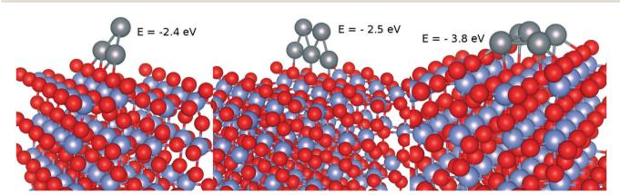
Fig. 4 Optimized geometries and binding energies of  $Ag_n$  clusters ( $n \le 5$ ) upon adsorption on the  $TiO_2(110)$  surface. Gray spheres represent silver atoms while red and blue spheres stand for oxygen and titanium atoms.
