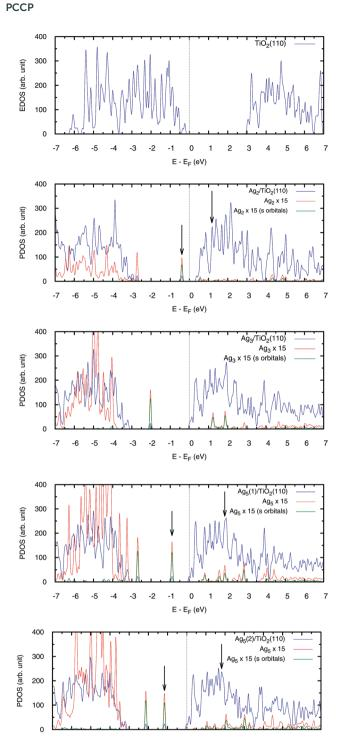
Fig. 5 EDOS of the  $TiO_2(110)$  surface and PDOS of the most stable  $Ag_n-TiO_2(110)$  systems obtained with the hybrid HSE06 functional, with  $Ag_5(1)$  and  $Ag_5(2)$  standing for the trapezoidal and pyramidal isomers (see Fig. 4). The zero of energy corresponds to the Fermi level, defined here as the highest occupied level. The arrows indicate the energies of the most responsible orbitals for the intense secondary peaks in the photoabsorption spectra (see Fig. 6).
