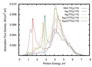
Fig. 6 Photo-absorption spectra of the  $TiO_2(110)$  surface, without adsorbates (shown in blue color) and with adsorbed  $Ag_n$  clusters. The most stable supported  $Ag_n$  clusters were considered, with  $Ag_5(1)$  and  $Ag_5(2)$  standing for the trapezoidal and pyramidal isomers (see Fig. 4). The arrows indicate the positions of the most intense secondary peaks across the near-infrared and visible regions of the solar spectrum.
