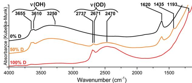
Fig. 4 IR spectra of the {001}-anatase-H<sub>2</sub>O sample dehydroxylated at 300 °C under flowing O<sub>2</sub>/Ar before (top) and after (bottom) isotopic exchange with D<sub>2</sub>O.
