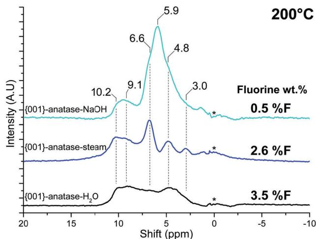
Fig. 11 NMR spectra of all the {001}-anatase samples at 200 °C. (A.U.: arbitrary units; \*: NMR bore contamination.)
