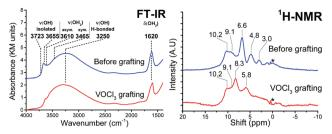
Fig. 12 FT-IR (left) and <sup>1</sup>H MAS SSNMR spectra of the {001}-anatasesteam sample dehydroxylated at 200 °C, before and after VOCl<sub>3</sub> grafting.
