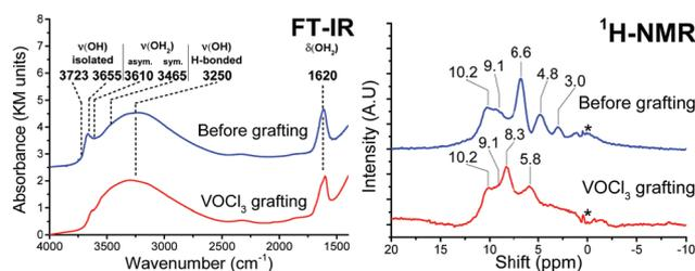
Fig. 12 FT-IR (left) and <sup>1</sup>H MAS SSNMR spectra of the {001}-anatase-steam sample dehydroxylated at 200 °C, before and after VOCl<sub>3</sub> grafting.
