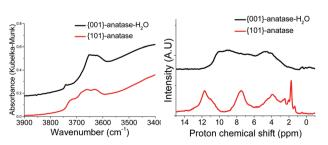
Fig. 3 DRIFTS (left) and  $^1$ H MAS SSNMR (right) spectra of the {001}-anatase and {101}-anatase samples after dehydroxylation at 300  $^\circ$ C.
