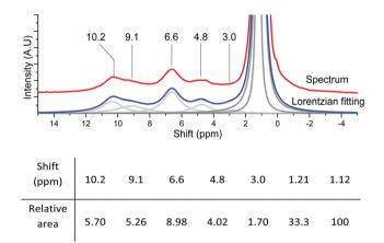
Fig. 13 Lorentzian fitting and relative areas of the fitted peaks of (001)-anatase-steam dehydroxylated at 200 °C with 1.23% adamantane.
