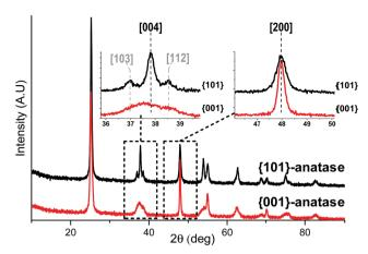
Fig. 1 X-ray diffractograms of the {001}-anatase-H<sub>2</sub>O and {101}-anatase samples.
