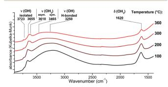
Fig. 5 DRIFTS infrared spectra of the  $\{001\}$ -anatase-steam sample after dehydroxylation at different temperatures. (Full data are available in the ESI,† Fig. S9.)
