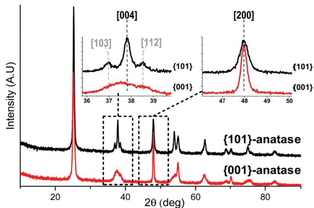
Fig. 1 X-ray diffractograms of the {001}-anatase-H<sub>2</sub>O and {101}-anatase samples.
