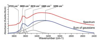
Fig. 6 In situ DRIFTS spectra of the  $\{001\}$ -anatase-steam sample at 300 °C (top) and its Gaussian fitting (bottom).
