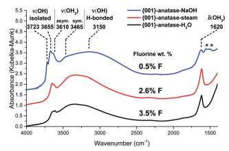
Fig. 8 DRIFTS infrared spectra of the  $\{001\}$  anatase-NaOH,  $\{001\}$  anatase-steam and  $\{001\}$ -anatase-H<sub>2</sub>O samples after dehydroxylation at 300 °C. (\*: carbonates contamination from NaOH.)
