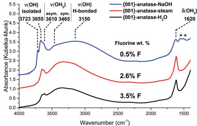
Fig. 8 DRIFTS infrared spectra of the {001} anatase-NaOH, {001} anatase-steam and {001}-anatase- $\text{H}_2\text{O}$  samples after dehydroxylation at  $300\text{ }^\circ\text{C}$ . (\*: carbonates contamination from NaOH.)
