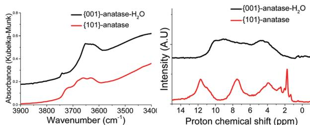
Fig. 3 DRIFTS (left) and <sup>1</sup>H MAS SSNMR (right) spectra of the {001}-anatase and {101}-anatase samples after dehydroxylation at 300 °C.
