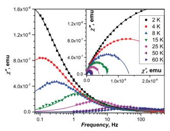
Fig. 8 Imaginary component of the magnetic susceptibility  $\chi''$  of non-diluted DySc<sub>2</sub>N@C<sub>80</sub> powder measured in zero field at selected temperatures. The inset shows Cole-Cole plots. Dots are experimental data points, lines are fits obtained with the generalized Debye model.
