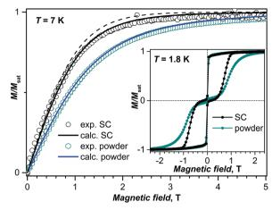
Fig. 4 Experimental (dots) and calculated (lines) magnetization curves of the powder and aligned single-crystal II (SC) of DySc<sub>2</sub>N@C<sub>80</sub> at T=7 K. Calculations for the single crystal took into account the presence of two crystallographic DySc<sub>2</sub>N sites in the crystal II (solid line); the dashed line is the calculated magnetization curve for the main site only. The inset shows magnetic hysteresis curves measured at 1.8 K for the powder and for the single crystal.
