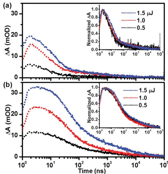
Fig. 4 Transient absorption kinetic decays of (a)  $\text{Fe}_2\text{O}_3$  and (b)  $\text{Fe}_2\text{O}_3\text{-SnTi}$  probed at 575 nm, as a function of excitation intensity (per pulse, 355 nm, 1 kHz); the inset shows normalized decays.
