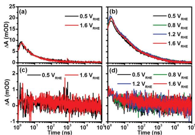
Fig. 5 Transient absorption kinetic decays of (a and c)  $\text{Fe}_2\text{O}_3$  and (b and d)  $\text{Fe}_2\text{O}_3\text{-SnTi}$  probed at (a and b) 575 and (c and d) 750 nm, as a function of applied bias following excitation at 355 nm ( $1 \mu\text{J}$  per pulse, 1 kHz).
