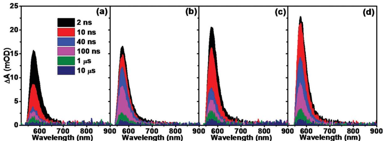
Fig. 2 Transient absorption spectra of (a) Fe<sub>2</sub>O<sub>3</sub>, (b) Fe<sub>2</sub>O<sub>3</sub>-Sn, (c) Fe<sub>2</sub>O<sub>3</sub>-Ti and (d) Fe<sub>2</sub>O<sub>3</sub>-SnTi following excitation at 355 nm (1  $\mu$ J per pulse, 1 kHz).
