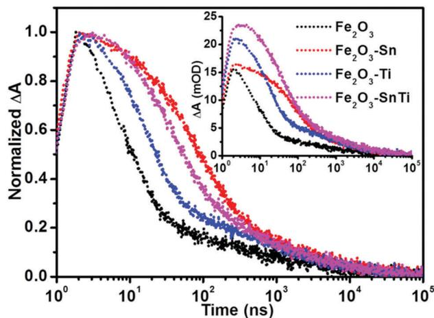
Fig. 3 Transient absorption kinetic decays of  $\text{Fe}_2\text{O}_3$ ,  $\text{Fe}_2\text{O}_3\text{-Sn}$ ,  $\text{Fe}_2\text{O}_3\text{-Ti}$  and  $\text{Fe}_2\text{O}_3\text{-SnTi}$  probed at 575 nm following excitation at 355 nm ( $1 \mu\text{J}$  per pulse, 1 kHz), the inset shows the kinetics before normalization.
