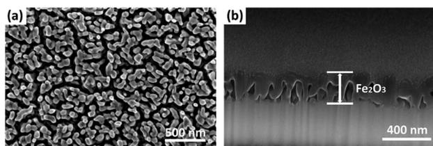
Fig. 1 SEM images of the Fe<sub>2</sub>O<sub>3</sub> film: (a) top view and (b) cross-sectional view.
