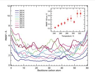
**Fig. 3** Root mean square fluctuations of PNIPAM backbone carbon atoms averaged over the last 75 ns of simulations. Results are shown for different temperatures. The inset displays the RMSF averaged over 100 ps, not including the first and last five residues of the chain. Errors are estimated by applying the blocking method.
