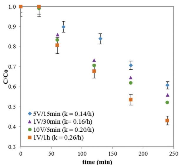
Fig. 4 SEM micrographs (top panel), nanowire diameter from statistical analysis of TEM micrographs (middle panel) and photocatalytic activity (bottom panel) for ZnO films obtained with 0.05 M  $\text{KHCO}_3$  at (a) 1 V/1 hour; (b) 10 V/5 min; (c) 1 V/30 min and (d) 5 V/15 min.
