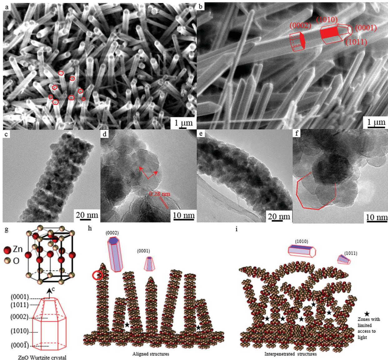
Fig. 7 SEM micrographs (anodization conditions: 0.1 M  $\text{KHCO}_3$  1 V/1 h) (top panel a and b), TEM micrographs (middle panel c–f) (anodization conditions 0.1 M  $\text{KHCO}_3$  1 V/1 h and 0.1 M  $\text{KHCO}_3$  5 V/15 min) and scheme of ZnO wurtzite-type crystals and ZnO nanowires (bottom panel g–i).
