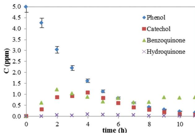
**Fig. 1** Photocatalytic degradation of phenol and formation of by-products. Error (%) for the by-products is similar to that of phenol (shown) but omitted for clarity.
