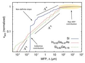
Fig. 5 Thermal conductivity accumulation function (TCAF) of natural Si,  $Si_{0.82}Ge_{0.18}$  and  $In_{0.53}Ga_{0.47}As$  at 300 K with  $L_{eff}$  = 7 mm.
