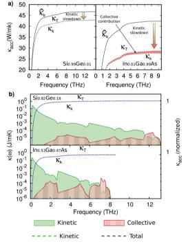
Fig. 2 (a) Thermal conductivity accumulation function (TCAF) for  $\mathrm{Si_{0.99}Ge_{0.01}}$  (left) and  $\mathrm{In_{0.01}Ga_{0.99}As}$  (right) for 7 mm rods at  $T=300~\mathrm{K}$ . (b) Thermal conductivity spectral distribution (TCSD) and TCAF in terms of frequency for  $\mathrm{Si_{0.82}Ge_{0.18}}$  (top) and  $\mathrm{In_{0.53}Ga_{0.47}As}$  (bottom) for 7 mm rods at  $T=300~\mathrm{K}$ .
