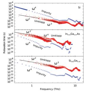
Fig. 6 Umklapp and impurity/alloy first principles relaxation times for Si, In<sub>0.53</sub>Ga<sub>0.47</sub>As and Si<sub>0.82</sub>Ge<sub>0.18</sub> at 300 K.
