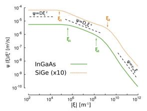
Fig. 3 Fractal diffusivity defined from  $\psi(\xi)/\xi^2$  for  $\ln_{0.53}\text{Ga}_{0.47}\text{As}$  and  $\text{Si}_{0.82}\text{Ge}_{0.18}$ .  $\text{Si}_{0.82}\text{Ge}_{0.18}$  curve is upscaled to ease the visualization. Three scaling regions with different exponents may be identified.
