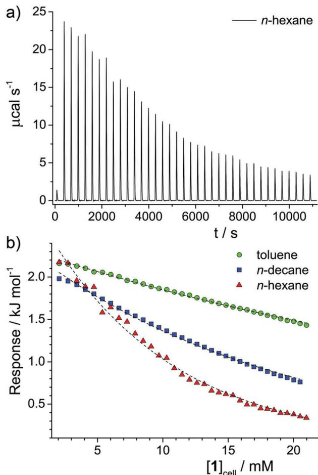
Fig. 3 (a) Raw data of recorded calorimetric response from repeated injections of a concentrated solution of **1** in *n*-hexane ( $[1] = 124 \text{ mM}$ ) into pure *n*-hexane. After an initial injection ( $1 \mu\text{L}$ ), each peak indicates a single injection of  $8 \mu\text{L}$ . (b) Plot of enthalpy change per mole of **1** injected versus the concentration of **1** in the sample cell,  $[1]_{\text{cell}}$ . Dashed lines are guides to the eye.
