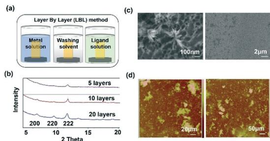
**Fig. 1** (a) LBL-D thin film preparation method for the SURMOF. (b) Thin film X-ray diffraction analysis of the prepared SURMOF, showing the increasing intensity of the  $2\theta$  value at  $11.6^\circ$  for (222) as the major face. (c) and (d) The SURMOF thin film surface was monitored by SEM and AFM, respectively, to confirm the particle size (nm scale) and the height. The SEM image showed the nanoporous surface of the MOF.
