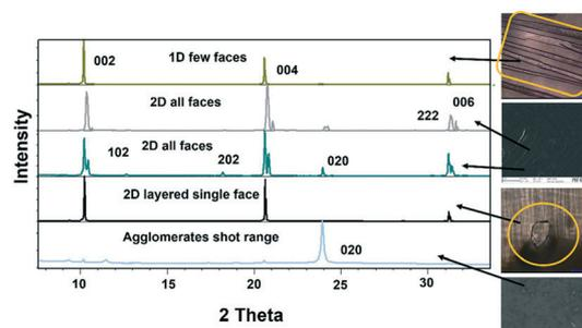
Fig. 4 Film XRD of the single crystals of form II, where a change in relative peak intensities was observed from needles to 2D crystals and agglomerates and spherical APAP molecules gave shot range  $2\theta$  at 24 for the (020) face. The top image on the right hand side is of the needles and the third one down is of the block crystals of form II.
