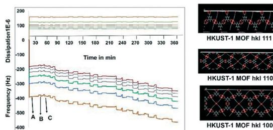
**Fig. 2** QCM-D adsorption and dissipation results of the metal, ligand and APAP. The results showed a change in frequency and dissipation with solution depositions of  $\text{Cu}(\text{OAc})_2$ , H3BTC and APAP. A–B–C, where A = Cu solution, B = H3BTC, C = APAP, and – = wash. The right hand side represents surface exposed highly porous MOF planes calculated from Materials Studio.
