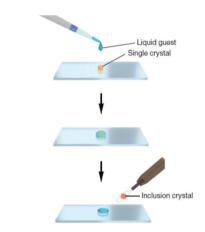
**Fig. 4** Preparation of a guest included network complex: a single piece of crystalline sponge is treated for 2 d (possibly under sealed conditions for volatile liquids) with a drop of a liquid guest and subjected to X-ray data collection (reproduced with permission from ref. 31).
