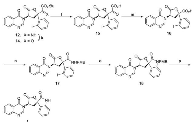
Scheme 8 (k) AcOH, THF/H<sub>2</sub>O, 73%; (l) TFA/CH<sub>2</sub>Cl<sub>2</sub>, quant; (m) Ph(OAc)<sub>2</sub>, AcOH/H<sub>2</sub>O, 80%; (n) PMBNH<sub>2</sub>, DIPEA, HATU, CH<sub>2</sub>Cl<sub>2</sub>/DMF, 70%; (o) CuI, Mg(OAc)<sub>2</sub>·4H<sub>2</sub>O, DMSO, 70%; (p) TfOH, CH<sub>2</sub>Cl<sub>2</sub>, 64%.
