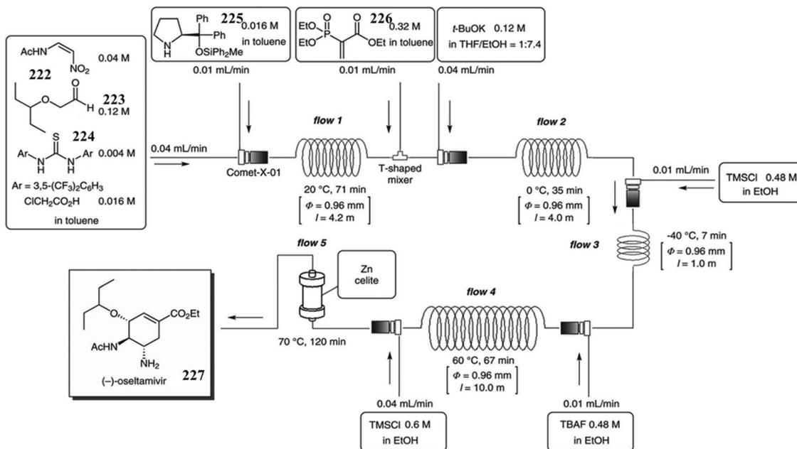
Fig. 27 Multi-step continuous flow synthesis of (-)-oseltamivir.
