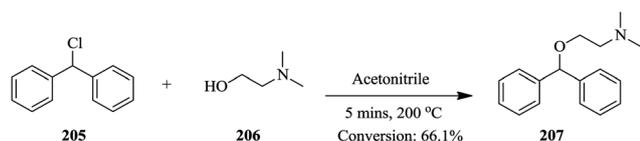
Scheme 40 Continuous flow synthesis of diphenhydramine.
