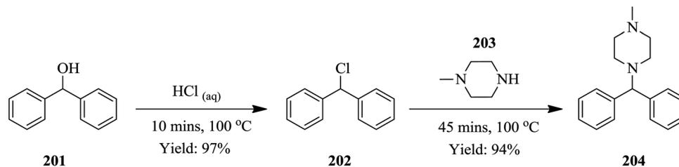
Scheme 39 A two-step continuous flow synthesis of cyclizine.
