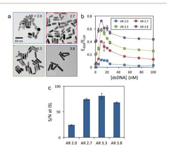
Fig. 2 Effect of AR of AuNRs on the assay performance. (a) TEM images of AuNRs with four different ARs. (b) Extinction coefficient ratio between 450 nm and LSP as a function of the 59 bp dsDNA concentration for the different AuNRs. All response curves have been offset for easier comprehension. (c) Signal-to-noise ratio (S/N) at the ISL for the different AuNR solutions.
