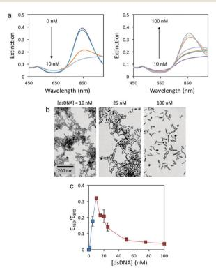
Fig. 1 Response of the colorimetric assay. (a) UV-Vis spectra of AuNRs with 3.8 AR in the presence of 0, 1, 5, 10, 15, 20, 25, 50, 75 and 100 nM 59 bp dsDNA. (b) TEM images of AuNRs in the presence of 10, 25 and 100 nM dsDNA. (c) Extinction ratio at 450 and 840 nm as a function of dsDNA concentration. The lower and higher concentration regimes are displayed in blue and red, respectively
