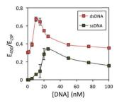
Fig. 4 Comparison between the response curves of single and double stranded DNA. AuNRs with an AR of 3.3 were used. All response curves have been offset for easier comprehension.
