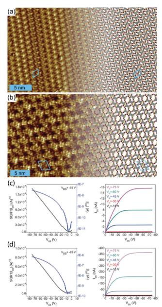
Fig. 2 Molecular packing observed at the TCB/HOPG interface for TB2TTA (a) and TB3TTA (b), together with indicative transfer (left) and output (right) characteristics for transistors made from TB2TTA (c) and TB3TTA (d) films. The STM parameters are  $l_t = 100$  pA and  $V_t = -800$  mV for (a) and  $l_t = 300$  pA and  $V_t = -450$  mV for (b). This figure is adapted from ref. 73 with permission from the Royal Society of Chemistry.
