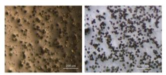
Fig. 1 Optical micrographs of single crystals of the {Np<sub>38</sub>} compounds synthesised from THF (1, left) and isopropanol (2, right).
