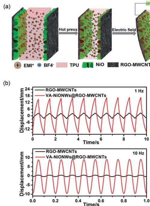
**Fig. 5** (a) Schematic illustration of the structure and assembly procedure of the actuators based on a hierarchically architected electrode. (b) Comparison of the bending performance of the actuators with and without vertically aligned NiO nanowires with an applied voltage of 2.5 V with frequencies of 1 Hz and 10 Hz. Figure is reproduced from ref. 65 with the permission of Royal Society of Chemistry.
