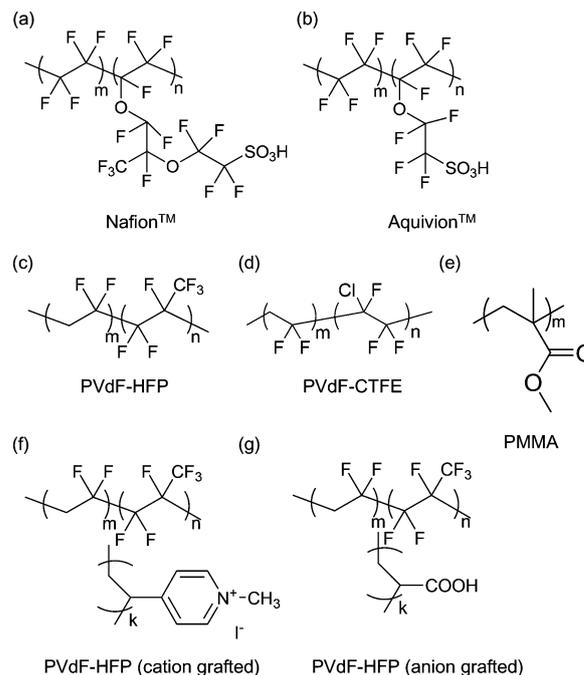
Fig. 2 Chemical structures of various polymers that have been employed for IPMC actuators: (a) Nafion<sup>TM</sup>, (b) Aquivion<sup>TM</sup>, (c) PVdF-HFP, (d) PVdF-CTFE, (e) PMMA, (f) cation-grafted PVdF-HFP, and (g) anion-grafted PVdF-HFP. (f) and (g) are reproduced from ref. 40 with the permission of American Chemical Society.
