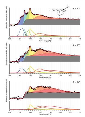
Fig. 3 Angle-dependence of NEXAFS from DCEDOT on Ag(111). The spectra (black points) are fit with a linear combination of peaks and a constant absorption edge.
