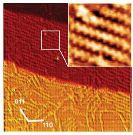
**Fig. 4** STM images of the annealed DCEDOT/Ag(111) surface (50 nm  $\times$  50 nm  $V_{\rm b}=-1.2$  V,  $I_{\rm t}=500$  pA). The white arrows indicate the inferred high-symmetry directions of the Ag(111) substrate. Zoomed inset shows details of the rows (7.1 nm  $\times$  7.1 nm).
