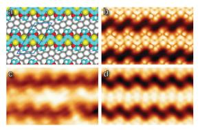
Fig. 5 (a) Model structure optimised by DFT. The unit cell is indicated with a blue outline. (b) Simulated STM image corresponding to the geometry in (a). (c) STM image ( $V_b = -1.2 \text{ V}$ ,  $I_t = 500 \text{ pA}$ ), and (d) simulated STM image with a Gaussian blur applied to simulate the finite radius of the STM tip. All images are 4.2 nm  $\times$  2.6 nm field of view.
