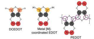
Fig. 1 Structure of DCEDOT, metal-coordinated EDOT, and PEDOT. The carbon atoms in each structure are color-coded. All structures contain B-carbon (gray) and ethylene-carbon (red). In the monomer, the  $\alpha$ -carbon (pink) is bonded to Cl, whereas in the metal-coordinated EDOT it is coordinated to a metal center (yellow), and in PEDOT it is bonded to a neighbouring EDOT monomer (purple open circles).
