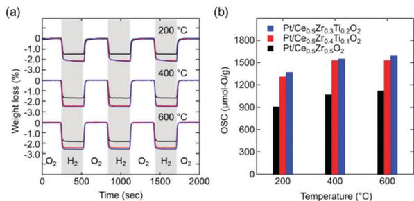
**Fig. 3** (a) TGA curves of Pt/Ce<sub>0.5</sub>Zr<sub>0.5-x</sub>Ti<sub>x</sub>O<sub>2</sub> upon switching between 5% O<sub>2</sub>/N<sub>2</sub> and 5% H<sub>2</sub>/N<sub>2</sub> every 5 min at various temperatures. (b) Estimated OSCs. Black, red, and blue lines and columns represent Pt/Ce<sub>0.5</sub>Zr<sub>0.5</sub>O<sub>2</sub>, Pt/Ce<sub>0.5</sub>Zr<sub>0.4</sub>Ti<sub>0.1</sub>O<sub>2</sub>, and Pt/Ce<sub>0.5</sub>Zr<sub>0.3</sub>Ti<sub>0.2</sub>O<sub>2</sub>, respectively.
