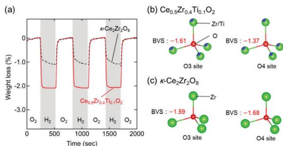
Fig. 5 (a) TGA curves of Pt/Ce<sub>0.5</sub>Zr<sub>0.4</sub>Ti<sub>0.1</sub>O<sub>2</sub> (black dashed line) and Pt/ $\kappa$ -Ce<sub>2</sub>Zr<sub>2</sub>O<sub>8</sub> (red solid line) during the atmosphere switching between 5% O<sub>2</sub>/N<sub>2</sub> and 5% H<sub>2</sub>/N<sub>2</sub> every 5 min at 200 °C. BVS values of the O3 and O4 sites in (b) Ce<sub>0.5</sub>Zr<sub>0.4</sub>Ti<sub>0.1</sub>O<sub>2</sub> and (c)  $\kappa$ -Ce<sub>2</sub>Zr<sub>2</sub>O<sub>8</sub>.
