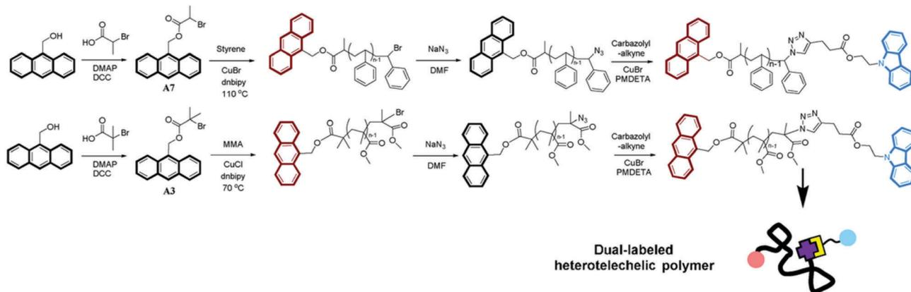
Fig. 6 Synthetic routes for  $\alpha,\omega$ -dye-functionalized PS and PMMA bearing anthryl and carbazoyl groups as FRET pairs. Anthryl moieties are first derivatized with ATRP initiating groups for the subsequent ATRP of styrene or methyl methacrylate, followed by chain end azidation and CuAAC with carbazoyl-alkyne. Adapted with permission from ref. 46.
