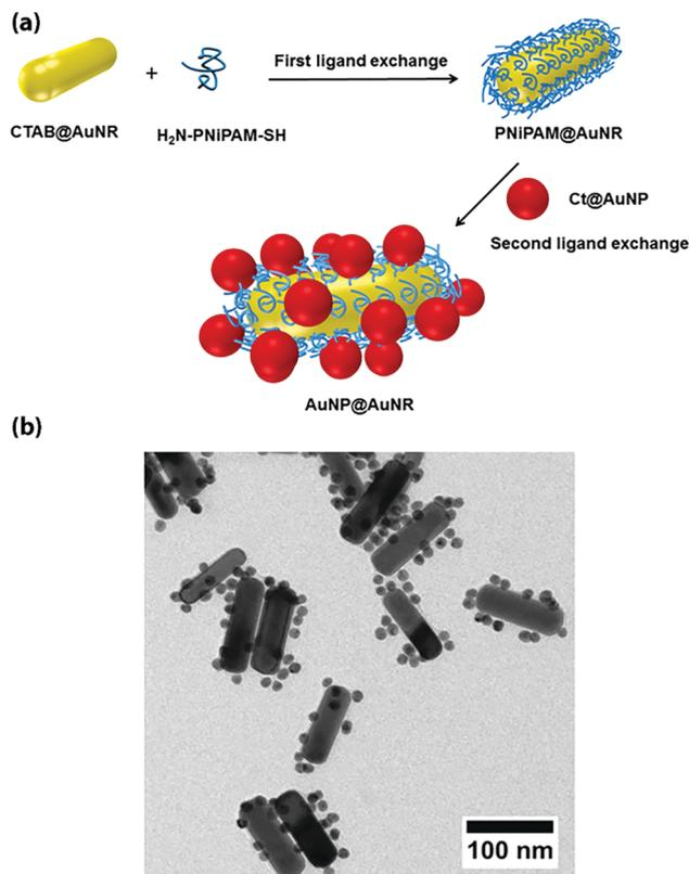
Fig. 15 (a) Linkage of heterotelechelic  $\alpha$ -amino,  $\omega$ -thiol PNIPAAm at the surface of AuNRs and further immobilization of AuNPs. (b) Transmission electron microscopy of AuNP@AuNR assembly. Adapted with permission from ref. 84.
