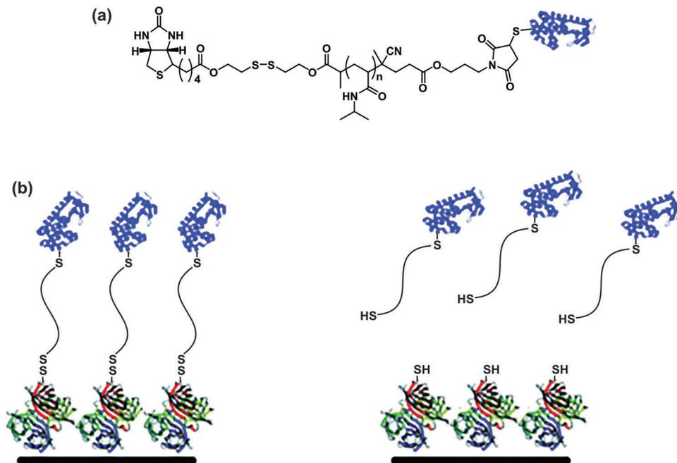
Fig. 12 (a) Structure of heterotelechelic  $\alpha$ -biotin,  $\omega$ -maleimide PNIPAAm containing a cleavable disulfide bond between the biotin and the polymer, after conjugation of BSA via thiol/maleimide linkage. (b) Immobilization of the conjugate via the biotin–SAv interaction and release from the surface by reduction of the disulfide bound. Adapted with permission from ref. 63.
