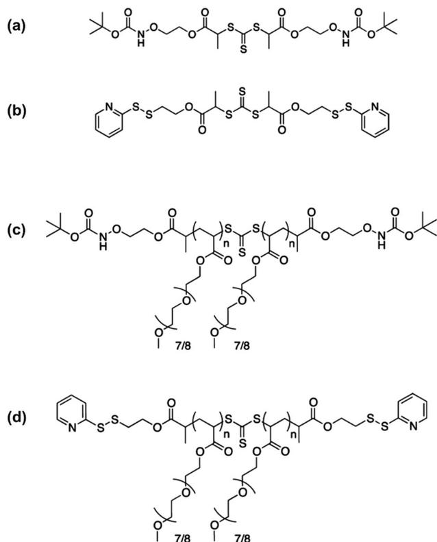
Fig. 8 Structure of difunctional, symmetric (a) *N*-Boc-aminooxy trithio-carbonate, (b) pyridyl disulfide trithiocarbonate, (c) telechelic *N*-Boc-aminooxy POEGA and (d) telechelic pyridyl disulfide POEGA. Adapted with permission from ref. 55.
