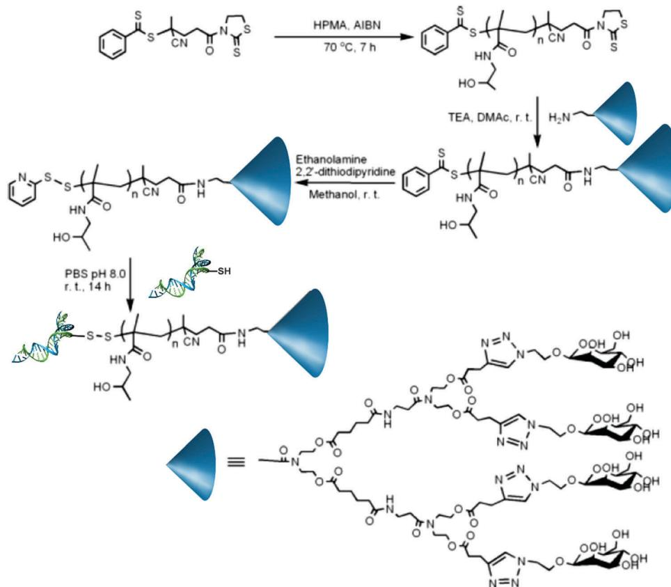
**Fig. 14** Synthesis of heterobifunctional siRNA–PPHMA–dendritic mannose biohybrid conjugates by RAFT polymerization of HPMA from a chain transfer agent bearing a 2-mercaptothiazolidine active ester group followed by coupling with dendritic-mannose G2Man on the  $\omega$  chain-end and with a short, thiolated interfering RNA on the  $\alpha$  position via disulphide bond formation after the reaction with a PDS moiety. Adapted with permission from ref. 67.
