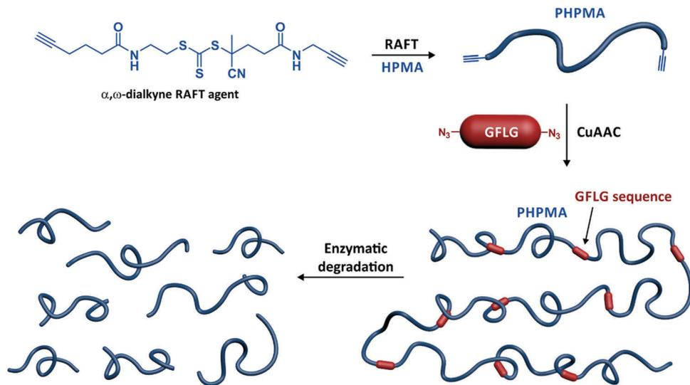
Fig. 5 Synthesis of multisegmented PHPMA by a combination of RAFT polymerization of HPMA from a  $\alpha,\omega$ -dialkyne trithiocarbonate chain transfer agent, followed by CuAAC between the resulting  $\alpha,\omega$ -dialkyne PHPMA and  $\alpha,\omega$ -diazide GFLG peptide sequence. Adapted with permission from ref. 33.
