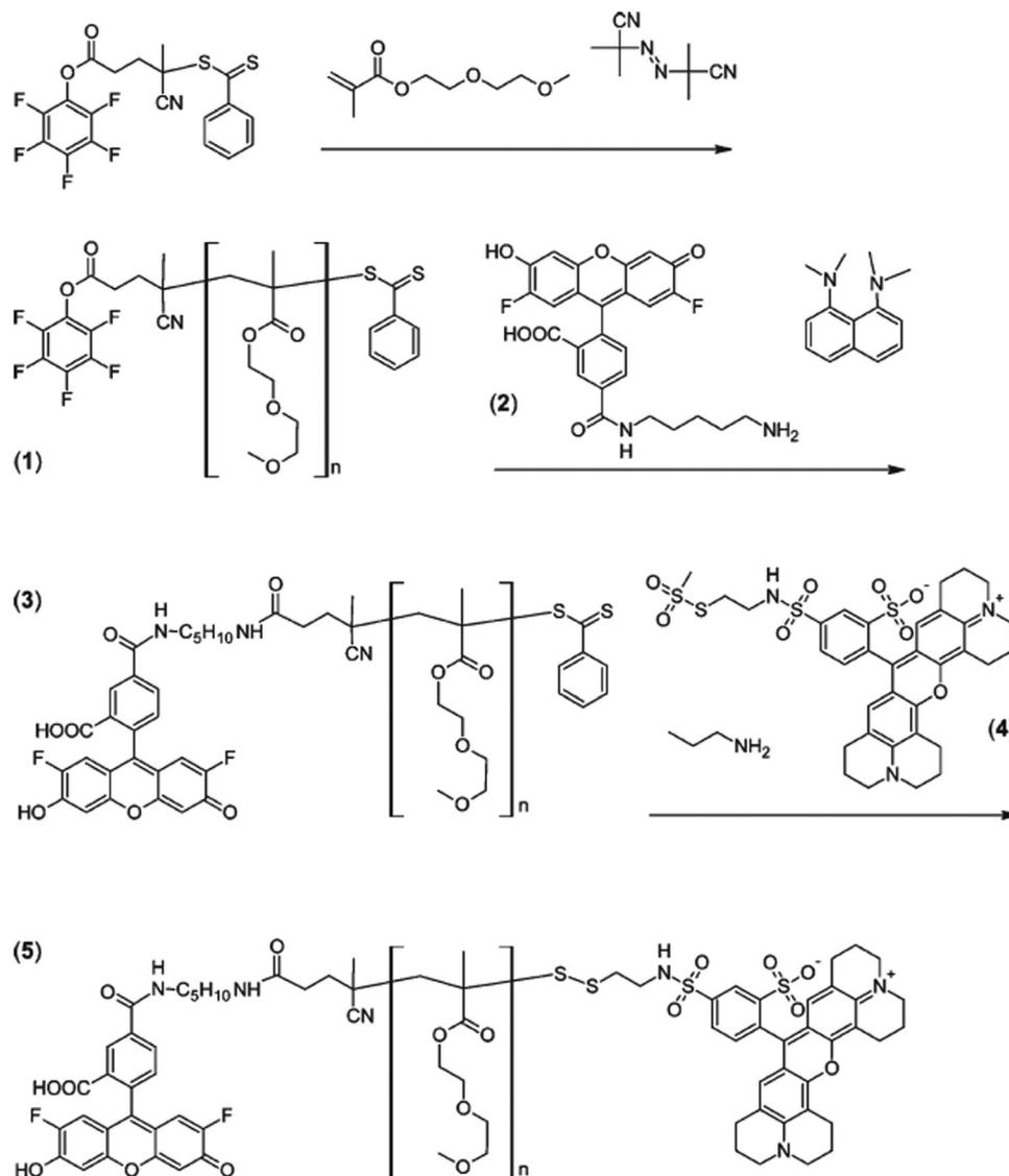
Fig. 7 RAFT synthesis of PDEGMA (1) from pentafluorophenyl activated ester RAFT followed by successive attachment of Oregon green cadaverin (2) by amidation on the  $\alpha$  position (3) and Texas red-2-sulfonamidoethyl methanethiosulfonate (4) by disulfide bond formation after aminolysis of the RAFT end group (5). Adapted with permission from ref. 47.
