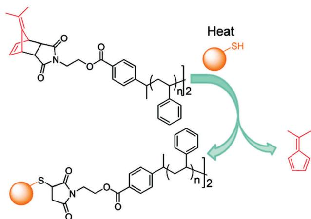
Fig. 9 Synthesis of a telechelic thiol-reactive polymer by ATRP and subsequent atom-transfer radical coupling, followed by conjugation to *N*-acetyl-L-cysteine methyl ester. Adapted with permission from ref. 56.
