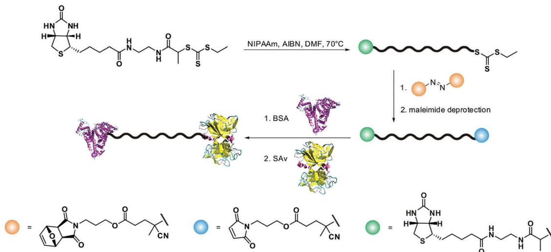
Fig. 10 Synthesis of heterotelechelic polymer–protein bioconjugates by RAFT polymerization of NIPAAm from a biotinylated chain transfer agent, followed by end-functionalization with a maleimide group and subsequent coupling with BSA *via* thioether bond formation and SAv *via* binding with biotin. Adapted with permission from ref. 53.
