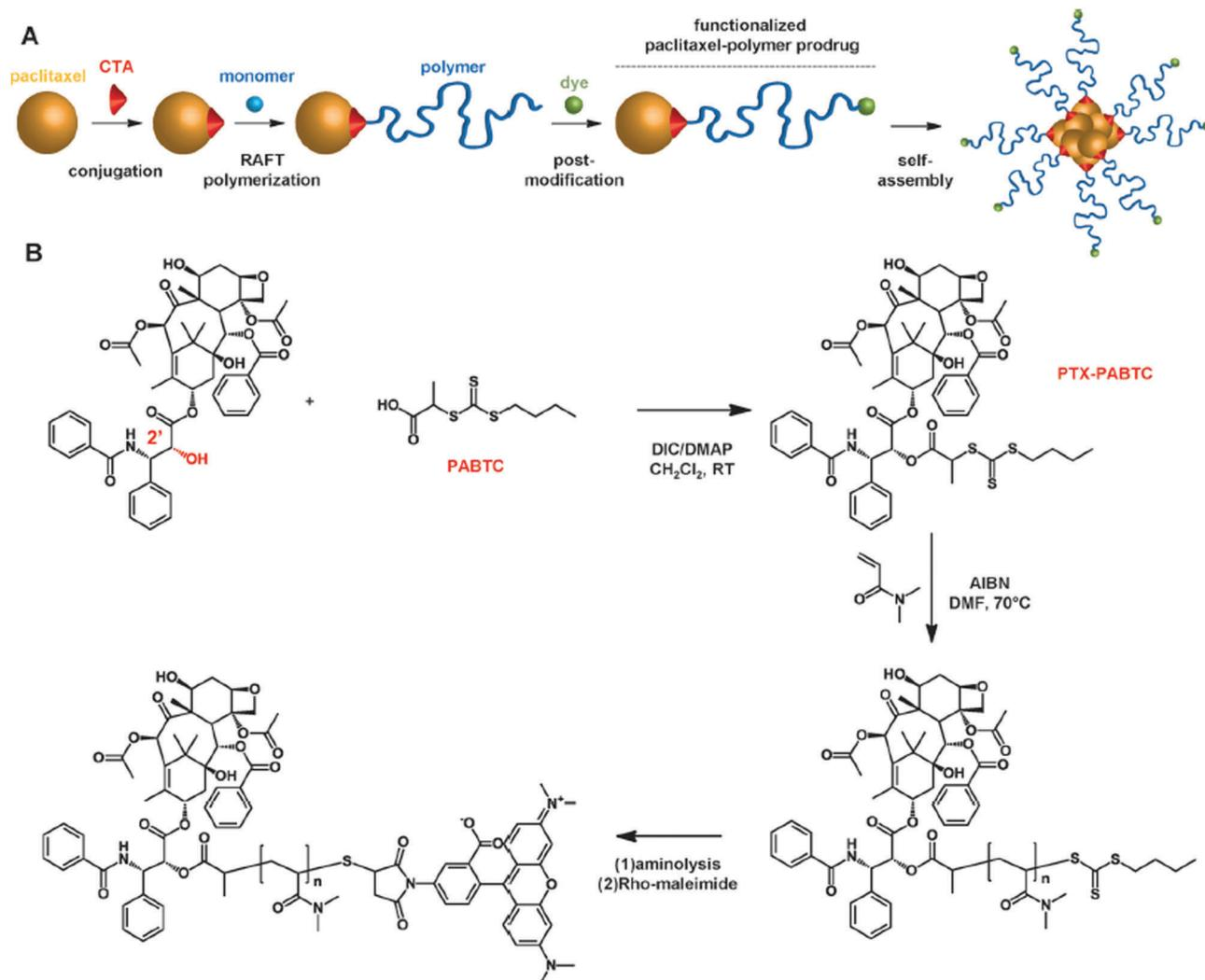
Fig. 4 (A) Synthesis of heterotelechelic  $\alpha$ -Ptx,  $\omega$ -rhodamine PDMA by RAFT polymerization from a Ptx-RAFT agent followed by a post-functionalization to link the fluorescent dye at the  $\omega$ -extremity and nanoprecipitation to yield the corresponding fluorescent polymer prodrug nanoparticles. (B) Synthetic strategy for the synthesis of heterotelechelic  $\alpha$ -Ptx,  $\omega$ -rhodamine PDMA. Adapted with permission from ref. 29.
