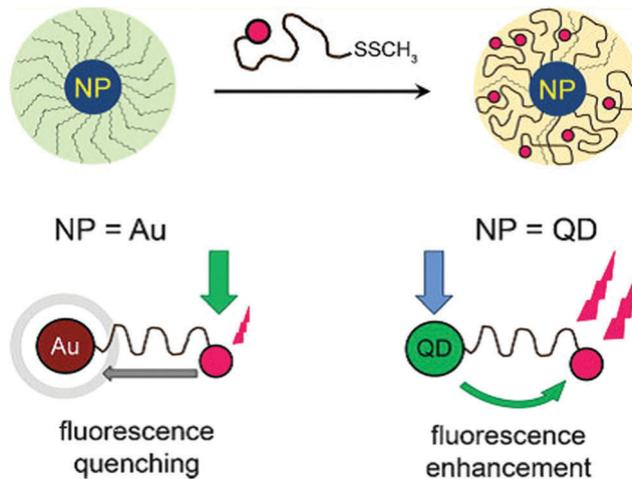
Fig. 17 Au nanoparticle or QD decoration by a heterotelechelic  $\alpha$ -dye,  $\omega$ -methyl disulfide poly(methyl methacrylate) and effect of the nearby Au core (fluorescence quenching) or QD (fluorescence enhancement) on the emission of the dye. Adapted with permission from ref. 92.
