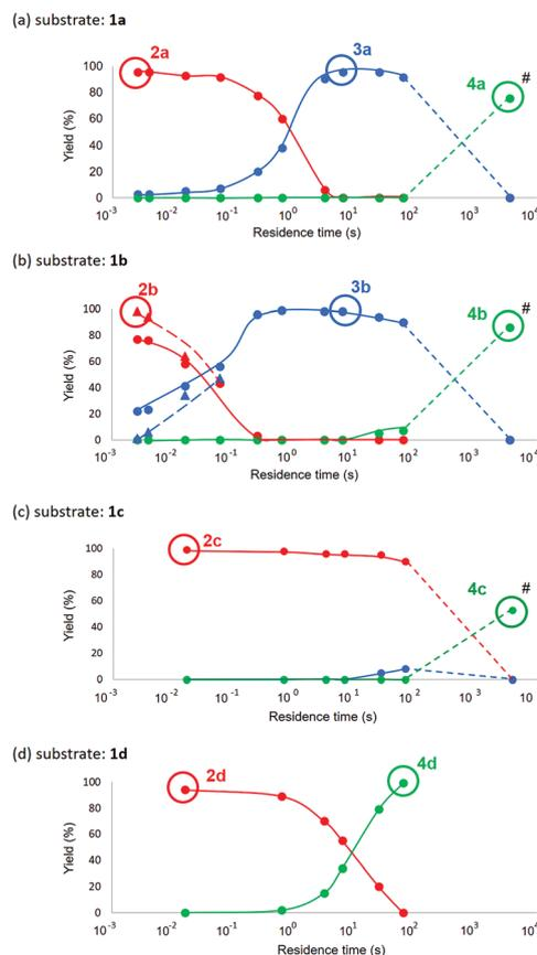
**Fig. 1** Tandem isomerizations of various aryl benzyl ethers by changing the residence time in R1 in a flow microreactor system for products **2**, **3** and **4d**, followed by further stirring in a flask at  $50\text{ }^{\circ}\text{C}$  for 1 h to obtain products **4a–c** (#). Methyl triflate was used as an electrophile (symbol  $\blacktriangle$  with a dashed line), instead of methyl iodide (symbol  $\bullet$  with a solid line).
