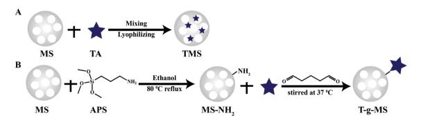
Scheme 1 Schematic diagram for the preparation of TA-loaded samples. (A) TMS prepared by simple physical adsorption. (B) T-q-MS as-synthesized utilizing glutaric dialdehyde to crosslink the amino group of MS-NH2 and the hydroxyl group of TA.
