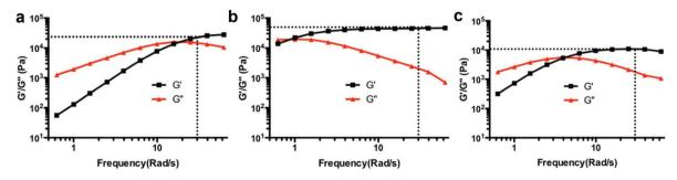
Fig. 2 Results of rheology frequency sweep test for hydrogels cross-linked with EGCG and EA at pH 7.4. (a) PEG4P-BA1-EGCG; (b) PEG8H-BA4-EGCG; (c) PEG8H-BA4-EA. G' and G'' represent storage and loss moduli, respectively. The storage moduli at 30 rad s<sup>-1</sup> are marked.
