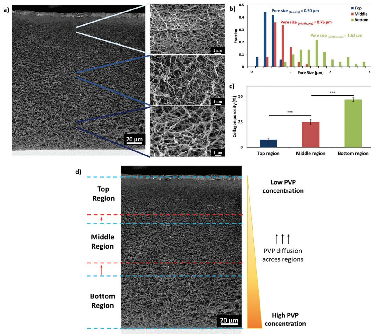
**Fig. 5** (a) FE-SEM images of representative bioprinted hierarchical porous collagen-based structures. Analysis of (b) pore size and (c) porosity of bioprinted collagen structures within the 3 different regions. (d) Printing accuracy according to the pre-defined hierarchical configuration; scale bar:  $20 \mu\text{m}$ .
