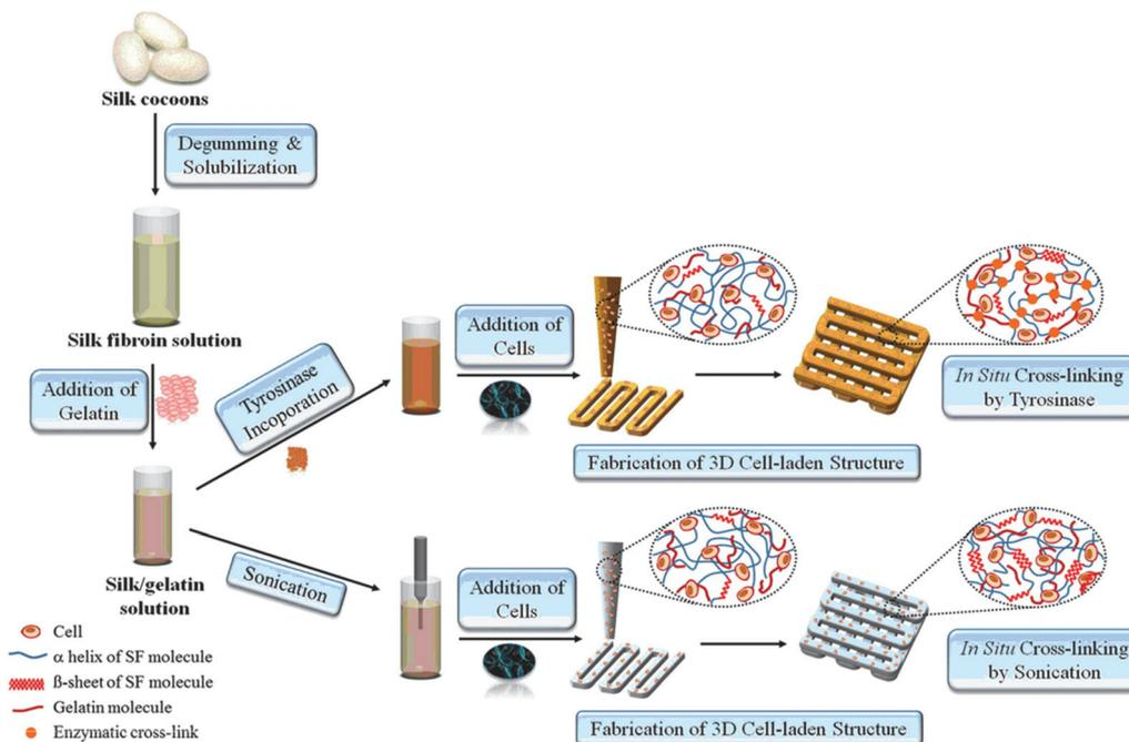
Fig. 3 The process of 3D-bioprinting of cell-encapsulated constructs by using silk-gelatin as a bioink.<sup>52</sup> Reprinted with permission Copyright Elsevier, 2014.
