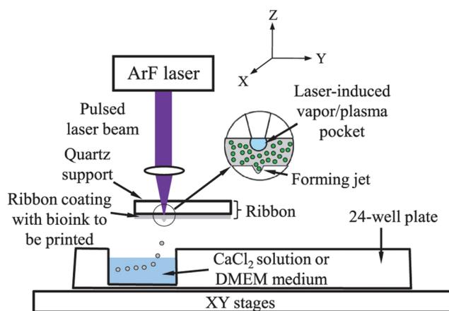
Fig. 5 Schematic representation of laser-assisted bioprinting.<sup>62</sup> Reprinted with permission Copyright IOP Publishing, 2014.
