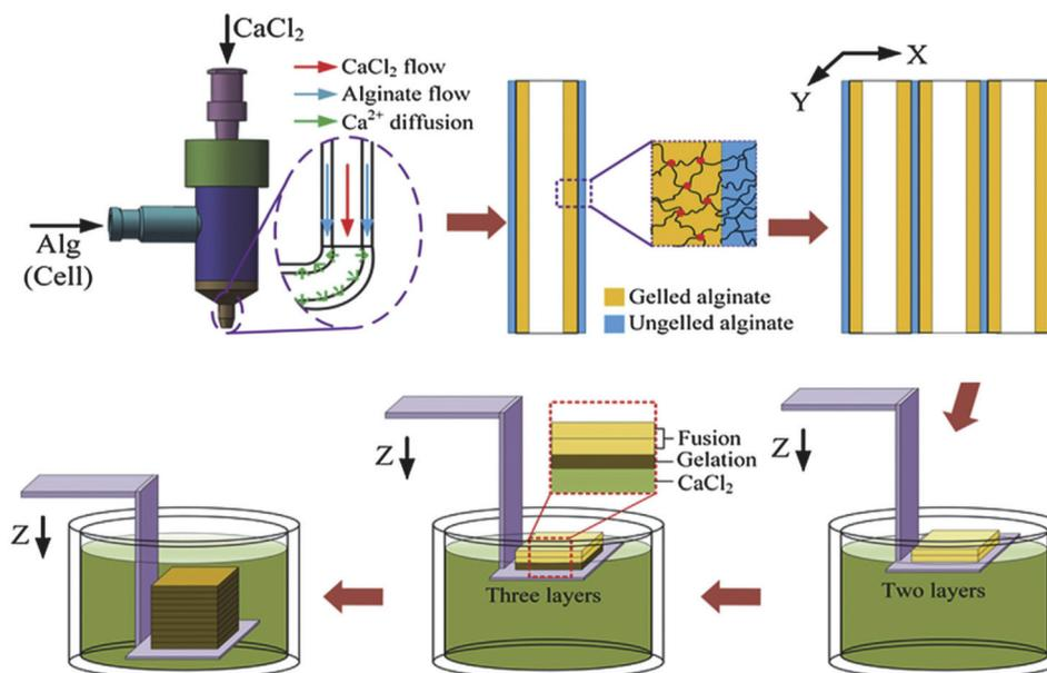
Fig. 4 Bioprinting process of a 3D structure with built-in microchannels by using an alginate bioink. Physical cross-linking process was utilized via calcium ions.<sup>61</sup> Reprinted with permission Copyright Elsevier, 2015.
