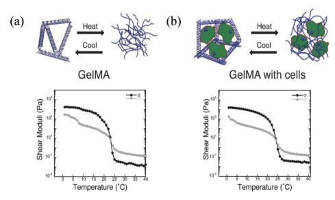
Fig. 2 Schematic diagrams of thermoresponsive gelation and the corresponding shear elastic (*G*') and loss moduli (*G*") measured as a function of temperature for: (a) pure GelMA, and (b) fibroblast-laden GelMA bioinks.<sup>39</sup> Reprinted with permission Copyright John Wiley & Sons, Inc., 2014.
