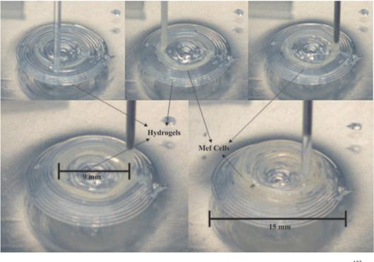
Fig. 14 Aggregate of MEF cells used as a bioink for bioprinting an aorta-like structure while the hydrogel served as a support. Reprinted with permission Copyright John Wiley & Sons, Inc., 2015.
