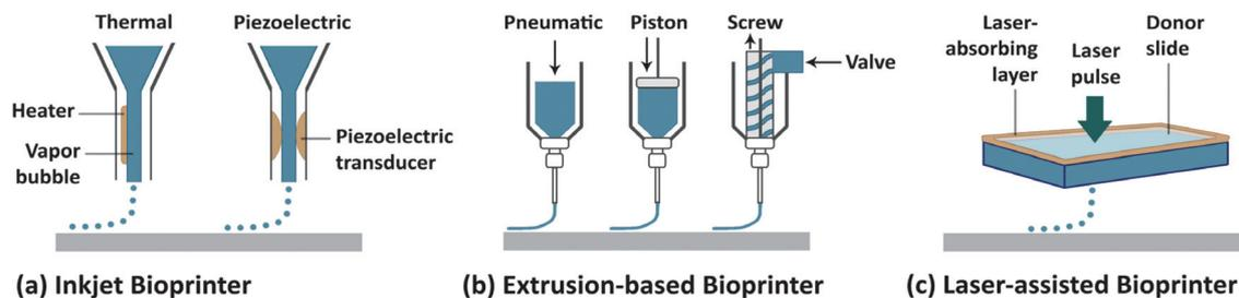
Fig. 1 Schematic representation of the main 3D bioprinting technologies. (a) Inkjet/droplet bioprinting. (b) Extrusion-based bioprinting. (c) Laser-assisted bioprinting.<sup>3</sup> Reproduced with permission Copyright Nature Publishing Group, 2014.
