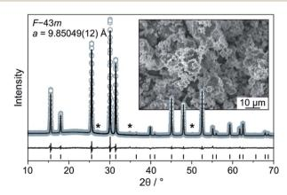
Fig. 1 Rietveld analysis of the XRD pattern for the  $\text{Li}_6\text{PS}_5\text{Cl}$  solid electrolyte. Asterisks denote impurities. The inset is a low-magnification SEM image of the as-prepared solid electrolyte powder.
