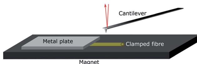
**Fig. 1** Custom-made sample holder to clamp fibres onto a hard surface in the AFM liquid cell. The fibres were clamped between a magnet glued into the liquid cell of the AFM and a metal slab with a thickness of 20  $\mu\text{m}$ .
