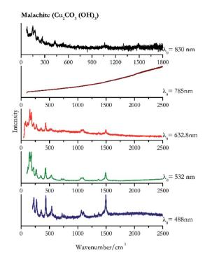
Fig. 24 Raman spectra of malachite
