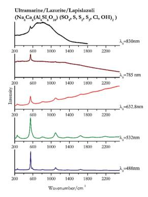
Fig. 16 Raman spectra of ultramarine.
