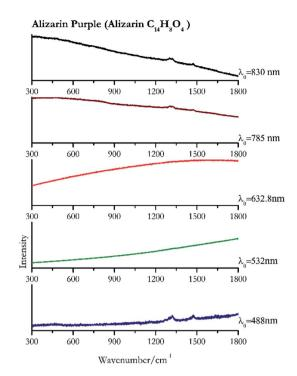
Fig. 12 Raman spectra of Alizarin purple.
