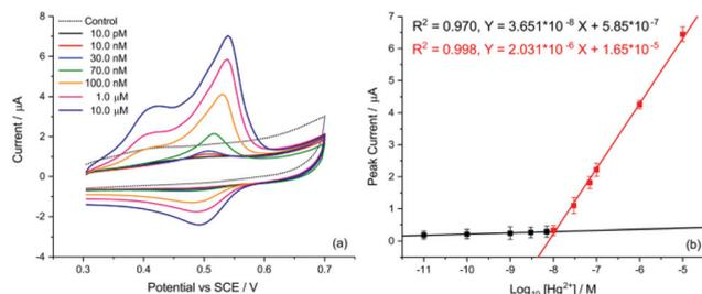
**Fig. 3** Detection of  $\text{Hg}^{2+}$  by CV. (a) Voltammograms of AuNP@TA-GCE at varying concentrations of  $\text{Hg}^{2+}$ . (b) Linear peak current behaviour at various  $\text{Hg}^{2+}$  concentrations.
