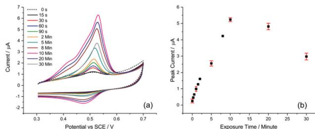
**Fig. 2** Assessment of electrode exposure times to  $1.0 \mu\text{M Hg}^{2+}$  by CV. (a) Voltammograms of AuNP@TA-GCE at various exposure times. (b) Current behaviour at peak-2 at exposures ranging from zero to 30 minutes.
