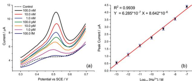
**Fig. 6** Detection of  $\text{Hg}^{2+}$  by SWV. (a) Voltammograms of AuNP@TA-GCE at varying concentrations of  $\text{Hg}^{2+}$ . (b) Linear peak current behaviour. Error bars represent relative standard deviation.
