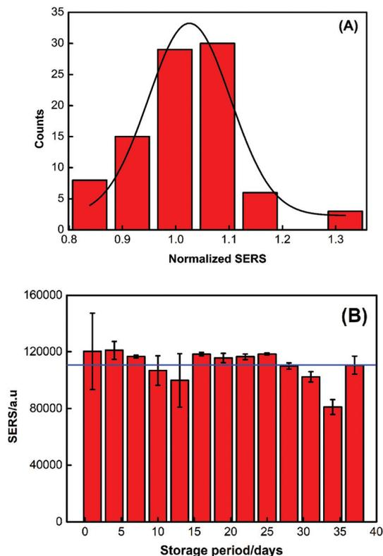
Fig. 4 (A) Statistics of a SERS mapping of a single PDMS sponge-SERS substrate. (B) SERS performance of 20  $\mu\text{L}$  100 nM R6G on the PDMS sponge-SERS substrate corresponding to different storage periods. The error bar shows the signal variation on a single substrate. Laser power: 10 mW. Integration time: 20 s. Objective: 20 $\times$ .
