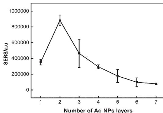
Fig. 3 SERS performance of different Ag NPs rounds-modified PDMS sponge. 10  $\mu\text{L}$  R6G (1  $\mu\text{M}$ ) was used as the Raman probe. Laser power: 14 mW. Integration time: 2 s. Objective: 20 $\times$ .
