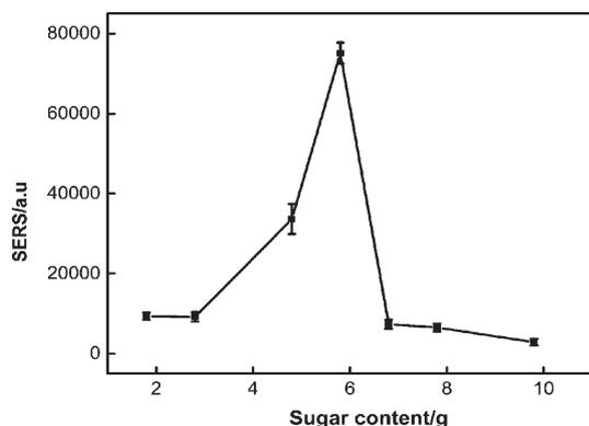
Fig. 2 SERS performance of Ag NPs-modified PDMS sponge prepared with varying amounts of sugar. A total of 10  $\mu\text{L}$  of R6G (1  $\mu\text{M}$ ) was used as the Raman probe. Laser power: 14 mW. Integration time: 2 s. Objective: 20 $\times$ .
