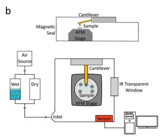
Fig. 1 (a) An illustrative representation of the main AFM-PTIR components is shown in the overhead configuration. (b) Schematic of the environmental chamber used for relative humidity studies: top panel-side view, and bottom panel-top view.
