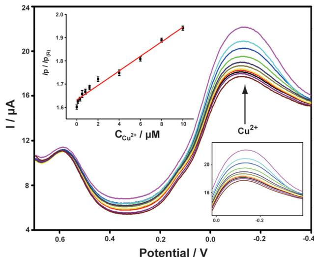
Fig. 3 DPV curves of the ABTS-PDDA/CNTs-NKB-GC toward successive additions of  $\text{Cu}^{2+}$  at the concentrations of 0, 0.1, 0.3, 0.5, 0.8, 1.2, 2.0, 4.0, 6.0, 8.0, and 10.0  $\mu\text{M}$ . The inset is the corresponding linear plot of the  $I_p/I_{p(R)}$  ratios versus the absolute concentrations of  $\text{Cu}^{2+}$ .
