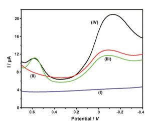
Fig. 2 DPV curves obtained on bare GC (I), PDDA/CNTs-GC (II), ABTS-PDDA/CNTs-GC (III) and ABTS-PDDA/CNTs-NKB-GC (IV) in the 100 mM PBS buffer solution containing  $8.0~\mu M Cu^{2+}$ .
