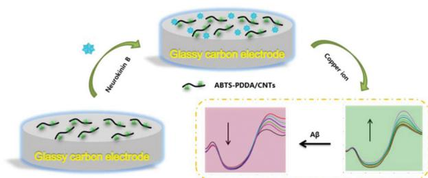
**Scheme 1** Combined determination of Cu<sup>2+</sup> and  $\beta$ -amyloid peptide based on the ratiometric ABTS-PDDA/CNTs-NKB biosensor.
