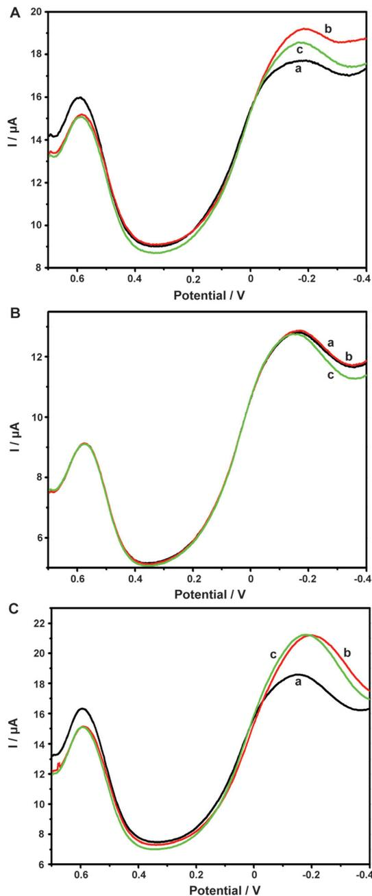
**Fig. 4** DPV curves obtained on ABTS-PDDA/CNTs-NKB-GC toward 1.8 (red curve, b) and 3.8  $\mu\text{g mL}^{-1}$   $\text{A}\beta_{1-42}$  (green curve, c) in the presence (A) and absence (B) of 6.0  $\mu\text{M}$   $\text{Cu}^{2+}$  PBS buffer. (C) The DPV responses of 10  $\mu\text{L}$  NaOH additions (b and c) to 6.0  $\mu\text{M}$   $\text{Cu}^{2+}$  PBS buffer.
