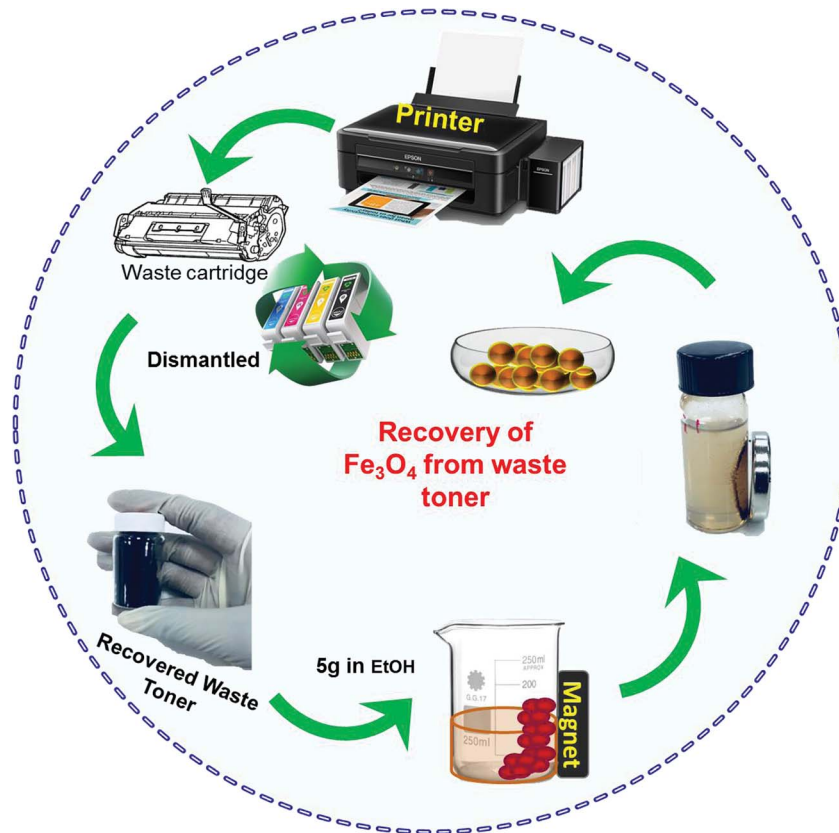
Scheme 1 Recovery procedure of \text{Fe}_3\text{O}_4 from the waste toner.
