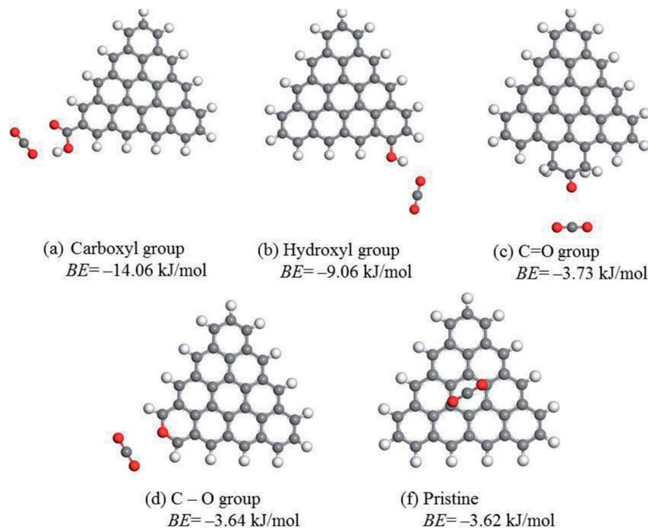
Fig. 5 Optimized geometries and the interaction of CO<sub>2</sub> with oxygen group-functionalized carbon.
