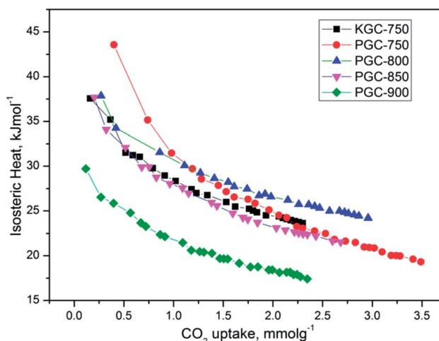
Fig. 6 Isothermic heat of adsorption as a function of CO<sub>2</sub> uptake.
