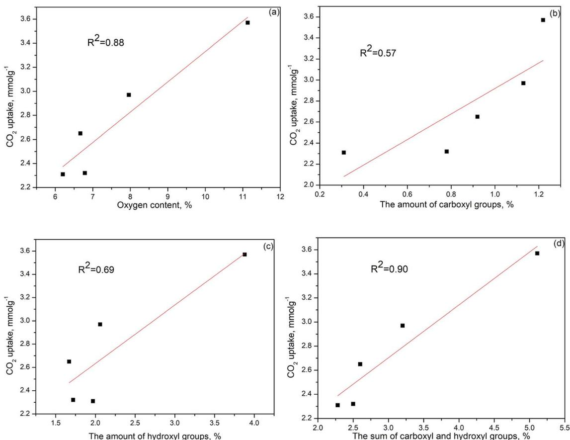
Fig. 4 Relationship between CO<sub>2</sub> uptake at 25 °C and surface chemistry of the as-prepared KC samples: (a) total oxygen content, (b) carboxyl groups, (c) hydroxyl groups, and (d) the sum of carboxyl and hydroxyl groups.
