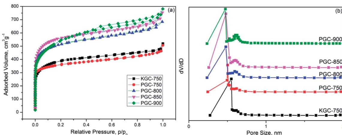
Fig. 2 Nitrogen adsorption/desorption isotherms and (a) pore size distribution (b) of the as-prepared samples.
