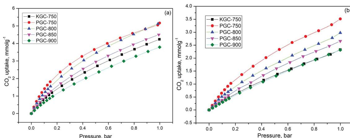
Fig. 3 CO<sub>2</sub> adsorption isotherms at (a) 0 °C and (b) 25 °C.
