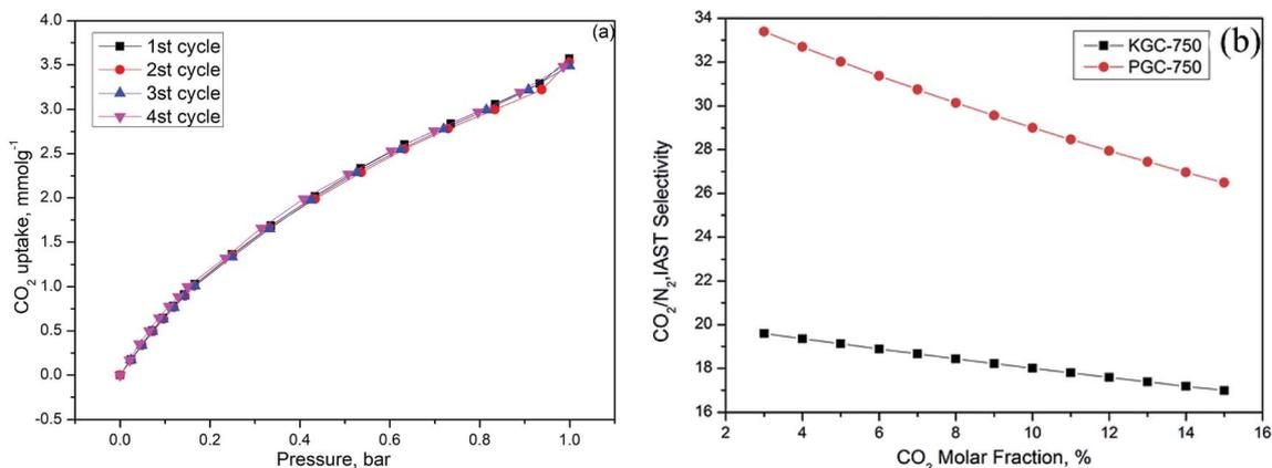
Fig. 7 (a) Regeneration performance of PGC-750, (b) CO<sub>2</sub>/N<sub>2</sub> selectivity of KGC-750 and PGC-750 as a function of CO<sub>2</sub> molar fraction.
