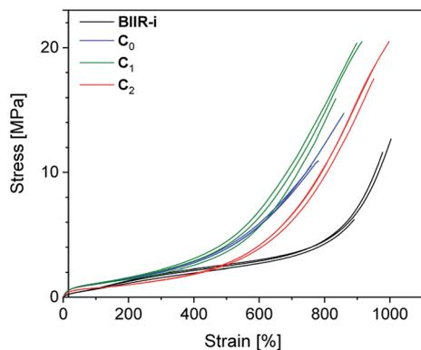
Fig. 8 Stress-strain curves of composites  $C_{0-2}$  compared to BIIR-i.
