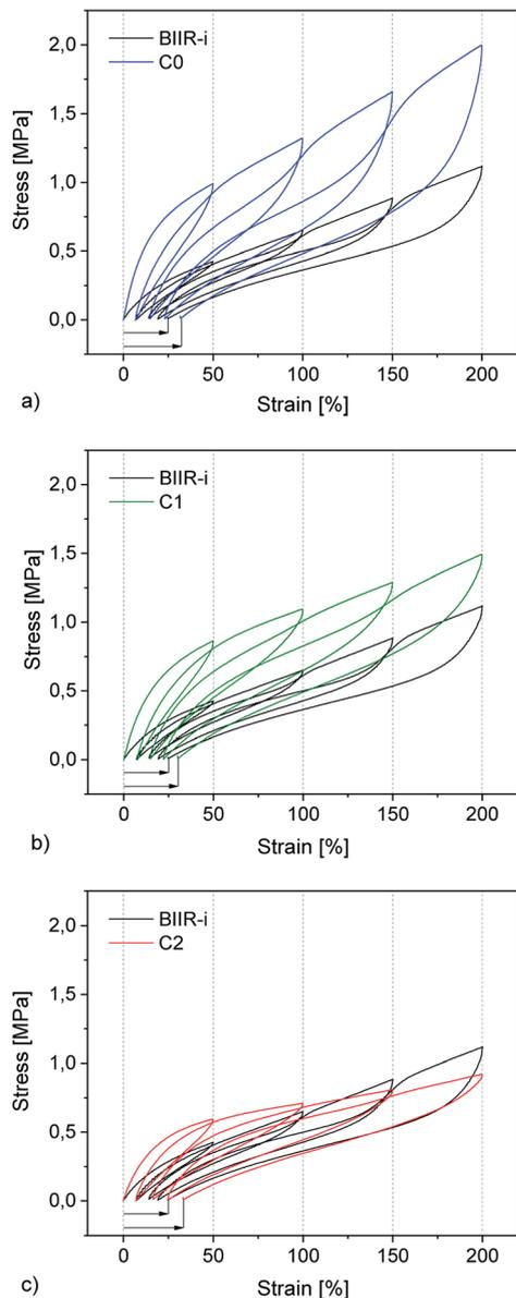
Fig. 7 Mechanical hysteresis curves of (a)  $C_0$ , (b)  $C_1$ , and (c)  $C_2$  in comparison to BIIR-i.
