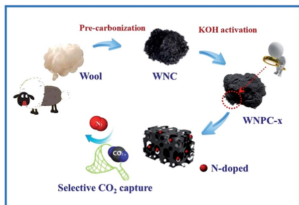
Fig. 1 Schematic illustrating the fabrication of WNPC-x and uses in selective CO 2 capture.
