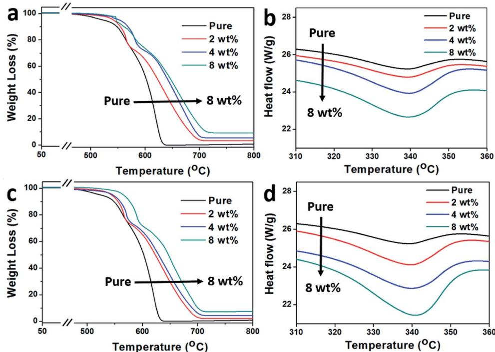
Fig. 7 TGA curves (a and c) and the corresponding DSC curves around the melting point (b and d) of the IF-WS<sub>2</sub>@C-30-PEEK and IF-WS<sub>2</sub>@C-60-PEEK composites, respectively.
