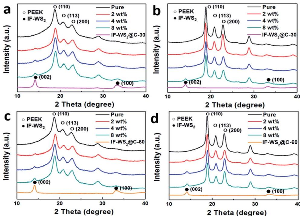
Fig. 2 XRD patterns of powdered mixtures of IF-WS<sub>2</sub>@C-PEEK before (a and c), and after (b and d) sintering crystallisation.
