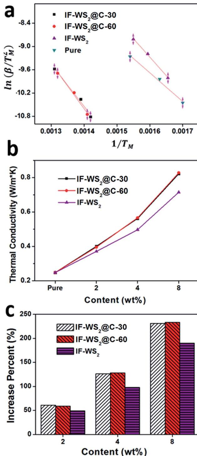
Fig. 8 (a) Determination of the activation energy using the Kissinger method for the neat PEEK, 8 wt% IF-WS<sub>2</sub>-PEEK and the 8 wt% IF-WS<sub>2</sub>@C-PEEK nanocomposites; (b and c) Thermal conductivity of the IF-WS<sub>2</sub>-PEEK and IF-WS<sub>2</sub>@C-PEEK nanocomposites against the neat PEEK.
