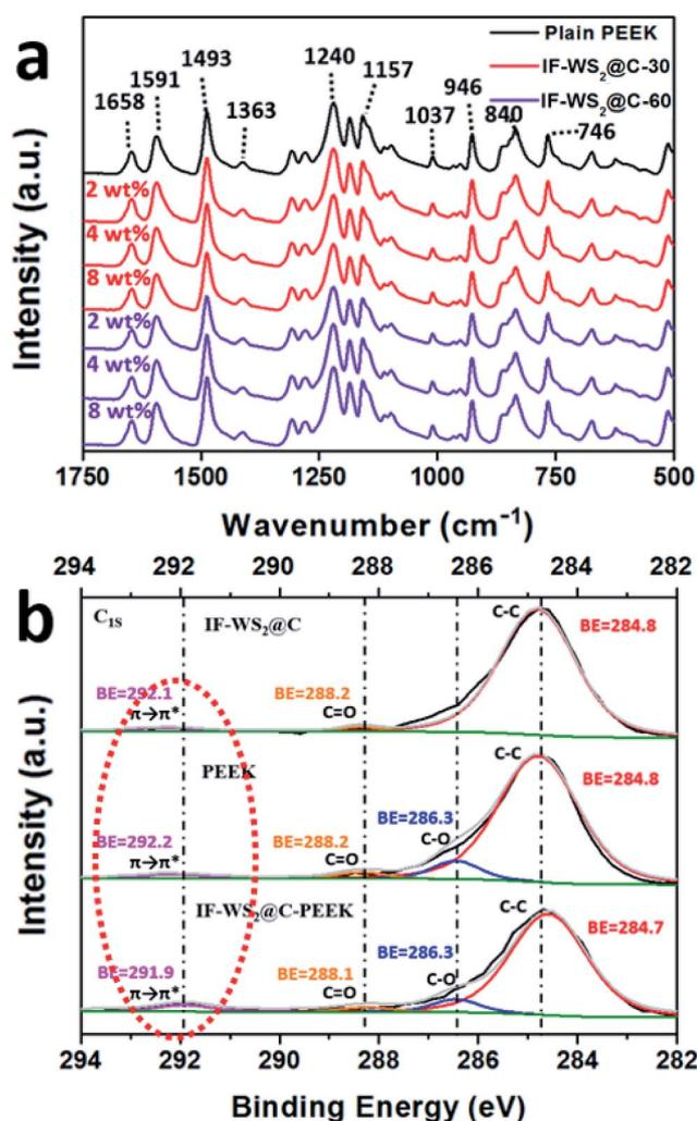
Fig. 5 (a) FTIR spectra and (b) XPS results of the C<sub>1s</sub> of the IF-WS<sub>2</sub>@C and its derived PEEK nanocomposites.
