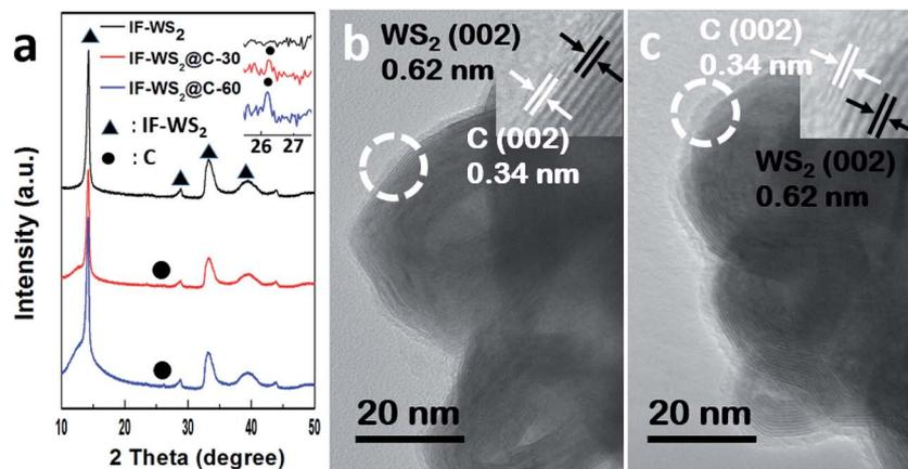
Fig. 1 (a) XRD patterns of pristine IF-WS<sub>2</sub> and IF-WS<sub>2</sub>@C NPs, with the inset showing the weak (002) peaks around 26°; (b and c) the HR-TEM images of IF-WS<sub>2</sub>@C-30 and IF-WS<sub>2</sub>@C-60 NPs.
