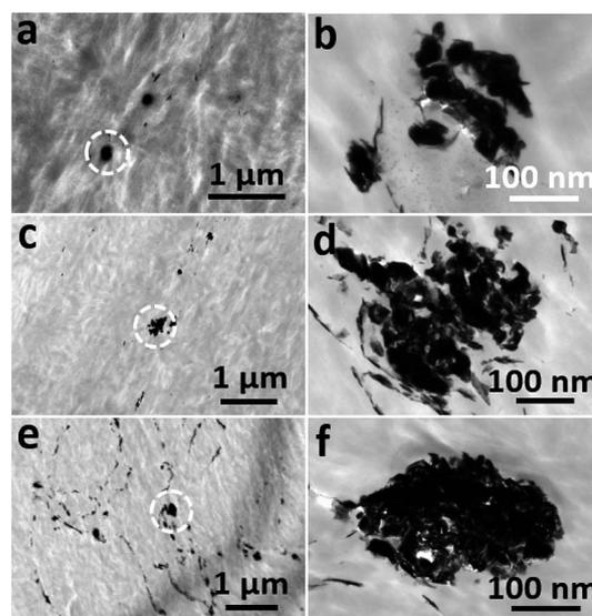
Fig. 4 TEM images of (a and b) 2 wt% IF-WS<sub>2</sub>@C-30-PEEK; (c and d) 2 wt% IF-WS<sub>2</sub>@C-60-PEEK and (e and f) 8 wt% IF-WS<sub>2</sub>@C-60-PEEK nanocomposites.
