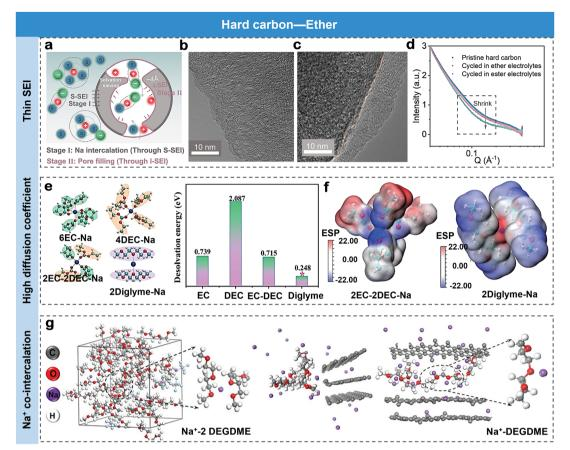
Fig. 8 Analysis of the critical role of ether in the HC of sodium batteries. (a)-(d) Thin SEI. Reproduced with permission, 149 Copyright © 2024, The Authors. (e) and (f) High Na<sup>+</sup> diffusion coefficient. Reproduced with permission, 150 Copyright © 2023, Tsinghua University Press. (g) Ether–Na<sup>+</sup> cointercalation. Reproduced with permission, 64 Copyright © 2021 Wiley-VCH GmbH.
