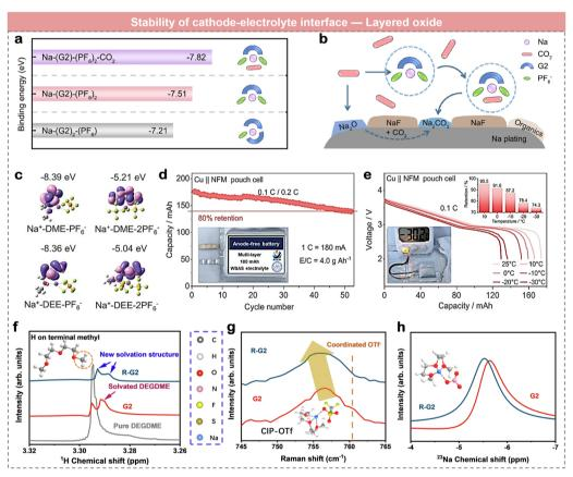
Fig. 11 Analysis of the critical role of ethers in layered oxide cathodes of sodium batteries. (a) and (b) CO2-regulated solvation structure. Reproduced with permission, <sup>172</sup> Copyright © 2023, American Chemical Society. (c)–(e) Weak solvent structure regulation. Reproduced with permission, <sup>167</sup> Copyright © 2024 Wiley-VCH GmbH. (f)-(h) Additive regulation. Reproduced with permission,<sup>175</sup> Copyright © 2025, The Authors.
