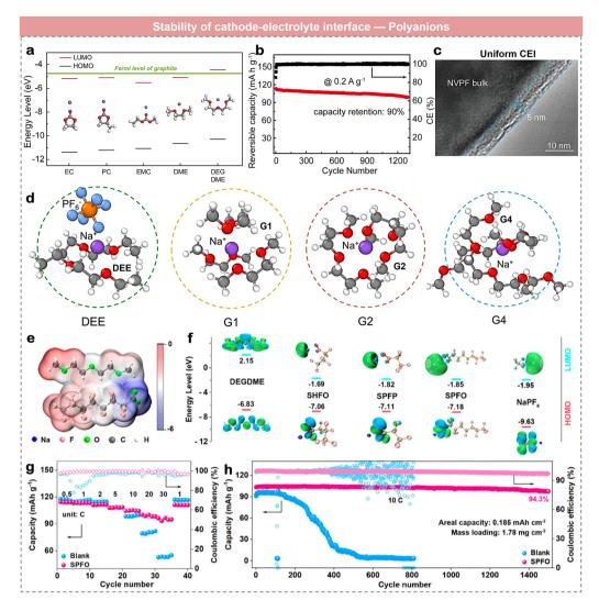
Fig. 12 Analysis of the critical role of ethers in polyanion cathodes of sodium batteries. (a)-(c) Salt concentration regulation. Reproduced with permission, 65 © 2021 Wiley-VCH GmbH. (d) Strong solvent structure regulation. Reproduced with permission, 170 Copyright © 2024 Elsevier B.V. (e)–(h) Additive regulation. 173 Reproduced with permission, Copyright © 2024, American Chemical Society
