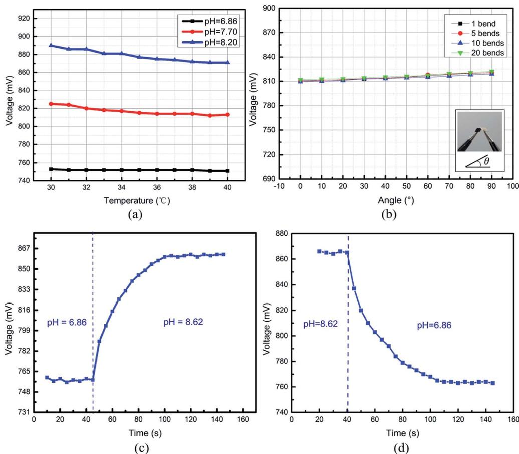
Fig. 7 (a) Flexibility experiments of the pH sensors. (b) Temperature effect of the pH sensors upon varying the temperature from  $30^\circ\text{C}$  to  $40^\circ\text{C}$  for three different pH levels. The dynamic response of the pH sensor for a step pH change shows (c) a rising time from pH 6.86 to 8.62 and (d) an inverse fall time from pH 8.62 to 6.86.
