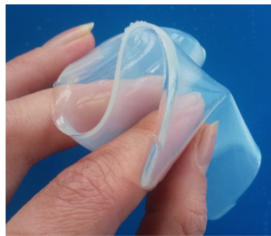
Fig. 11 Demonstrative flexibility of cellulose hydrogel.
