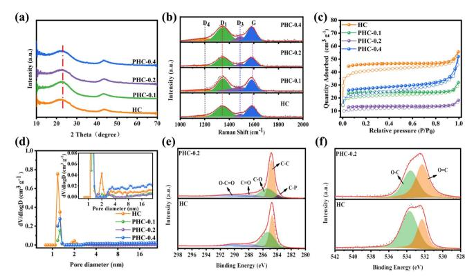
Fig. 1 (a) XRD patterns; (b) Raman spectra; (c) N<sub>2</sub> adsorption/desorption isotherms; (d) pore size distribution; (e) C 1s spectra; (f) O 1s spectra.
