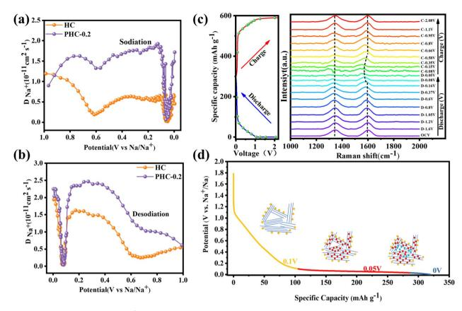
Fig. 5 For the PHC-X anode: (a and b) Na<sup>+</sup> diffusion coefficients during the discharge process and charge process. (c) *In situ* Raman spectra and the corresponding discharge—charge profiles at the first cycle of PHC-0.2 for SIBs. (d) Schematic diagram of the sodium storage stages of hard carbon.
