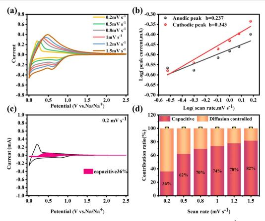
Fig. 4 For the PHC-0.2 electrode: (a) cyclic voltammetry curves at different scan rates between 0.2 and 1.5 mV s<sup>-1</sup>, (b) the plots of  $\log(i)$  versus  $\log(v)$ , (c) pseudocapacitive contribution at 0.2 mV s<sup>-1</sup>, and (d) pseudocapacitive contribution at different scan rates between 0.2 and 1.5 mV s<sup>-1</sup>.
