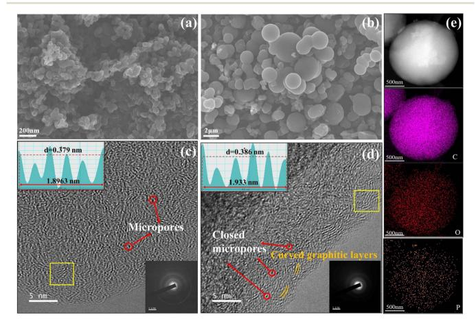
Fig. 2 SEM images of (a) HC and (b) PHC-0.2; HRTEM images and lattice distance of (c) HC and (d) HC-0.2. Inset shows the corresponding SAED and FFT patterns. (e) STEM based element mapping of PHC-0.2.
