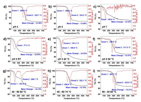
Fig. 2 DSC profiles of the MFP precursors synthesized at different reaction conditions, indicating the onset decomposition temperature and the mass change for (a-c) different pH values, (d-f) different reaction temperatures, and (g-i) different Mn to Fe ratios.
