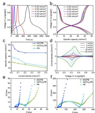
Fig. 4 Electrochemical performances of PB, Ni(OH)<sub>2</sub>/PB, and NiO/PB. a, (b) GCD curves of NiO/PB at different current densities. (c) Specific areal capacities of PB, Ni(OH)<sub>2</sub>/PB, and NiO/PB at different current densities. (d) CV curves of NiO/PB under various sweep rates. Nyquist plots of PB, Ni(OH)<sub>2</sub>/PB, and NiO/PB (e) before and (f) after cycling.
