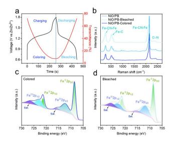
Fig. 6 (a) GCD curves at current densities of 0.1 mA cm<sup>--2</sup> and simultaneous transmittance (@632.8 nm) evolution. (b) Raman spectra of NiO/PB in various states (original, colored, and bleached). High-resolution XPS spectra of Fe 2p in NiO/PB at (c) colored and (d) bleached
