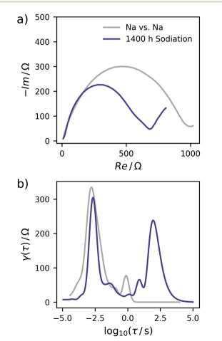
Fig. 3 (a) Nyquist plot of the symmetrical Na/Na cell. (b) DRT of the symmetrical cell. Data of the C-HAT-1600 anode is shown for comparison.
