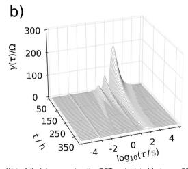
Fig. 8 Waterfall plot comparing the DRTs calculated between 50 h and 350 h. In (a) experimental data are depicted, (b) shows DRTs calculated from simulated data assuming the model described in Fig. 7.
