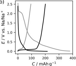
Fig. 1 (a) Ar physisorption isotherm at 87 K. (b) Galvanostatic chargedischarge curves recorded at 18.6 mA h g<sup>-1</sup>. The first cycle (grey) and representative capacity-limited cycle (black) is depicted, respectively.
