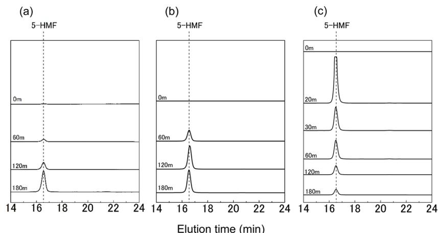
Fig. 3 GPC chromatograms of ChCl/glucose DES after heating at 100 °C (a), 130 °C (b), 160 °C (c) for various treatment times. Detector: PDA UV 280 nm.
