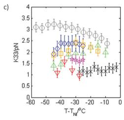
**Fig. 9** The splay,  $K_{11}$  (a), twist,  $K_{22}$  (b) and bend,  $K_{33}$  (c) elastic constants as a function of  $T - T_{\rm NI}$  for compound **1** (black crosses), compound **2** (grey circles), mixture 1 (red downward triangles), mixture 2 (green upward triangles), mixture 3 (blue diamonds), mixture 4 (oranges squares) and mixture 5 (magenta stars).
