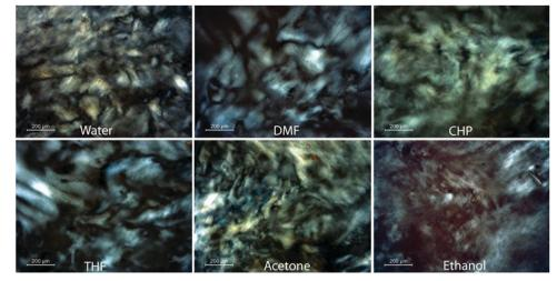
Fig. 5 Schlieren textures observed in dispersions of graphene oxide in a range of organic solvents under microscopy using crossed polarisers. Reproduced with permission from Jalili et al., ACS Nano, 2013<sup>78</sup> (©2013 American Chemical Society).
