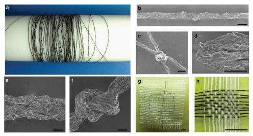
Fig. 7 (a) Four-metre-long wound GO fibre. SEM images of the fibre (b), and a typical tighten knot (c). (d) The morphology of the GO fibre after tensile tests. All scale bars 50 μm. Reproduced with permission from Xu and Gao, Nat. Commun., 2011<sup>4</sup> (©2011 Nature Publishing Group).
