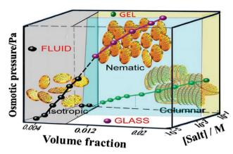
Fig. 4 Phase diagram of graphene oxide agueous dispersions in terms of osmotic pressure, volume fraction of GO and salt concentration in the solution. Reproduced with permission from Konkena and Vasudevan, J. Phys. Chem. C, 2014<sup>75</sup> (©2014, American Chemical Society).
