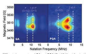
Fig. 3 EPR nutation spectra of QA and PQA (T = 10 K) oxidized with 1 eq. per arylamine unit. The microwave power was set so  $f^{\circ}(S = 1/2) = 7.7$  and 4.4 MHz for QA and PQA (respectively).
