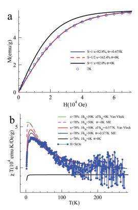
Fig. 4 (a) Magnetization of QA diluted in a polystyrene matrix (0.58%<sub>mol</sub>) versus magnetic field at T = 2 K. (b) Product of magnetic susceptibility and temperature ( $\chi T$ ) vs. temperature at H=5000 Oe obtained for the **QA** sample diluted in a polystyrene matrix (see the ESI,† Section VIII for expression used for the Van Vleck eqn (S3) and the magnetization eqn (S4), derived from the Heisenberg exchange Hamiltonian).
