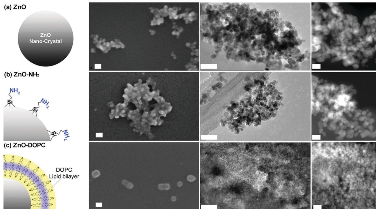
Fig. 1 The three ZnO nanocrystals used in this study: (a) pristine ZnO NCs, (b) amine-propyl functionalized ZnO-NH<sub>2</sub> NCs, and (c) lipid-coated ZnO-DOPC NCs. From left to right: scheme of the particles, FESEM, TEM and STEM images for each NC type. For FESEM images all the NCs were coated by a thin layer of Pt. The scale bar is 50 nm in all FESEM and TEM images, whereas it is 20 nm in all the three STEM images (right column).
