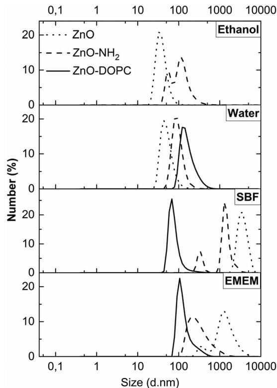
Fig. 4 Dynamic Light Scattering (DLS) measurements in number % of the ZnO samples, pristine ZnO NCs (dotted curves), ZnO-NH<sub>2</sub> NCs (dashed curves), and ZnO-DOPC NCs (solid curves) in different media (ethanol, water, SBF, and EMEM).
